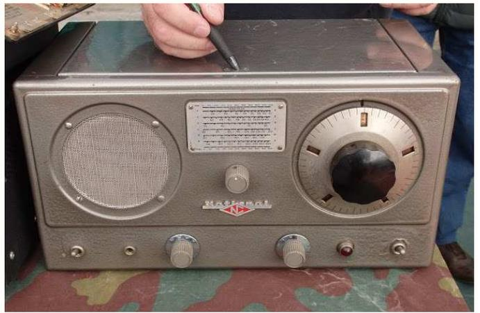
**Ricevitore National HFS (VHF)** da 27 a 250 MHz (A: 178-250 MHz, B: 120-178 MHz, C: 80-120 MHz, D: 56-80 MHz, E: 41-60 MHz, F: 27-42 MHz nei modi AM, CW, FM
